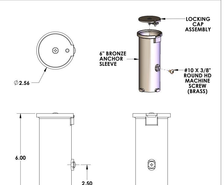
THE SCOUT ANCHOR INCLUDES A 6" DEEP BRONZE ANCHOR SLEEVE, A BRONZE LOCKING CAP WITH A BRONZE LOCKING BAR AND A #10 X 1/2" STAINLESS STEEL MACHINE SCREW, AND A #10 X 3/8" BRASS ROUND-HEAD SCREW FOR BONDING. THE SLEEVE WILL ACCOMODATE A  $\emptyset$  1.9" DIAMETER X 6" LONG POST.
