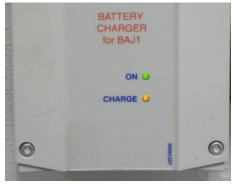
B. When the battery is correctly installed on the charger or control box you should hear a "click" indicating the battery is properly seated on the unit. Also note that when the battery is properly seated there should not be any gaps between the battery and the control box/charger.
