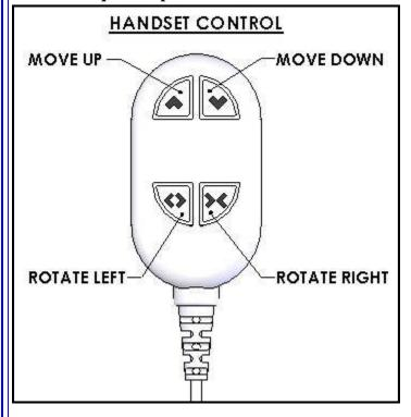
lift UP, press the top left button with the ▲ symbol and hold it down until the lift has reached its desired height and then release the button. The other buttons work in a similar fashion. In all cases, releasing the button will cause the lift to stop moving.
