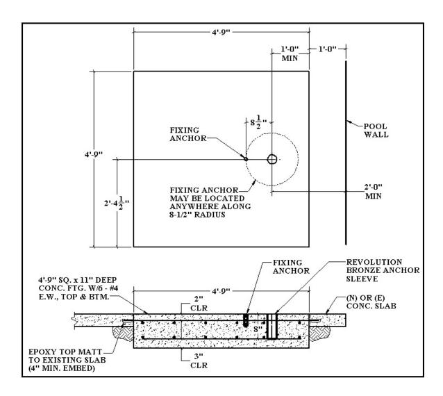
NOTE: For the SLING OPTION the maximum setback distance (from the pool wall to the anchor) is 24".
